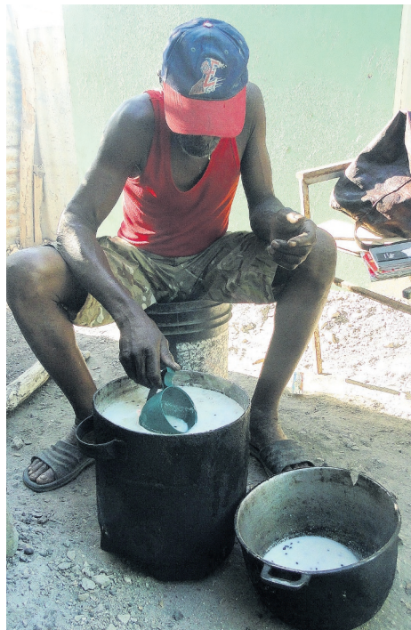
Lewie Foster removing the first-stage formation of castor oil into another pot.
