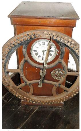
A clock used to record working hours.
